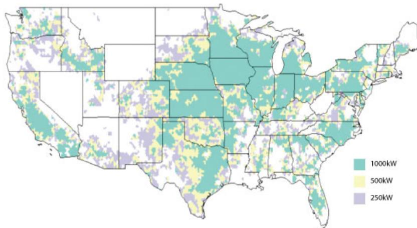
Readily available manure resources can contribute over 11 000 MW of electricity generation potential. Each colored grid cell can support an anaerobic digester of a given capacity.
