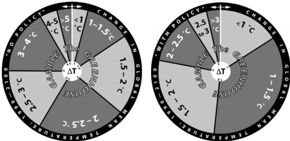
Figure 2. The probabilities for various amounts of global average warming between 1990 and 2100 calculated from two multi-hundred sets of model forecasts are projected onto two wheels. 3 The left-hand wheel is for “no policy” and the right-hand wheel is for “policy” (see text).
