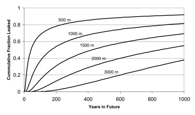
Figure 1. Leakage over time as a function of injection depth.
