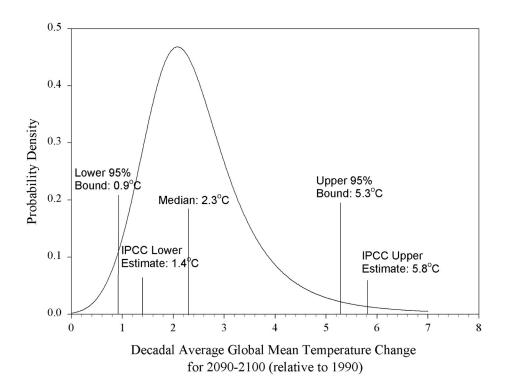
Probability density function for the change in global-mean surface temperature from 1990 to 2100, estimated as a best-fit of a beta distribution to 100 simulations using Latin Hypercube sampling from input distributions. The IPCC upper estimate is beyond our 95% confidence limit. Based on this distribution, there is a 12% chance that the temperature change in 2100 would be less than the IPCC lower estimate.
