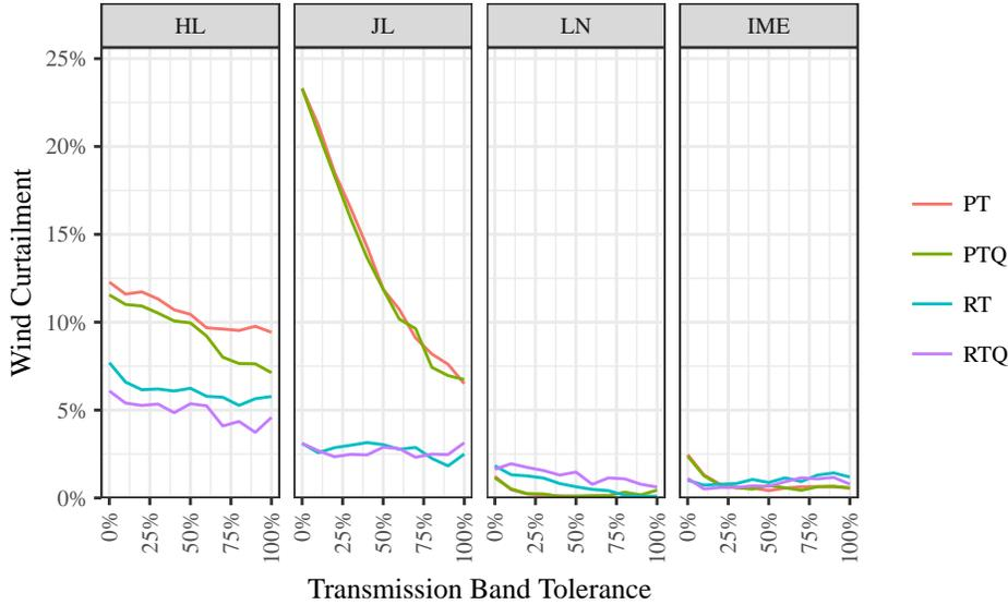
Figure 5.12: Curtailment by province for transmission band tolerance sensitivity, Northeast.
