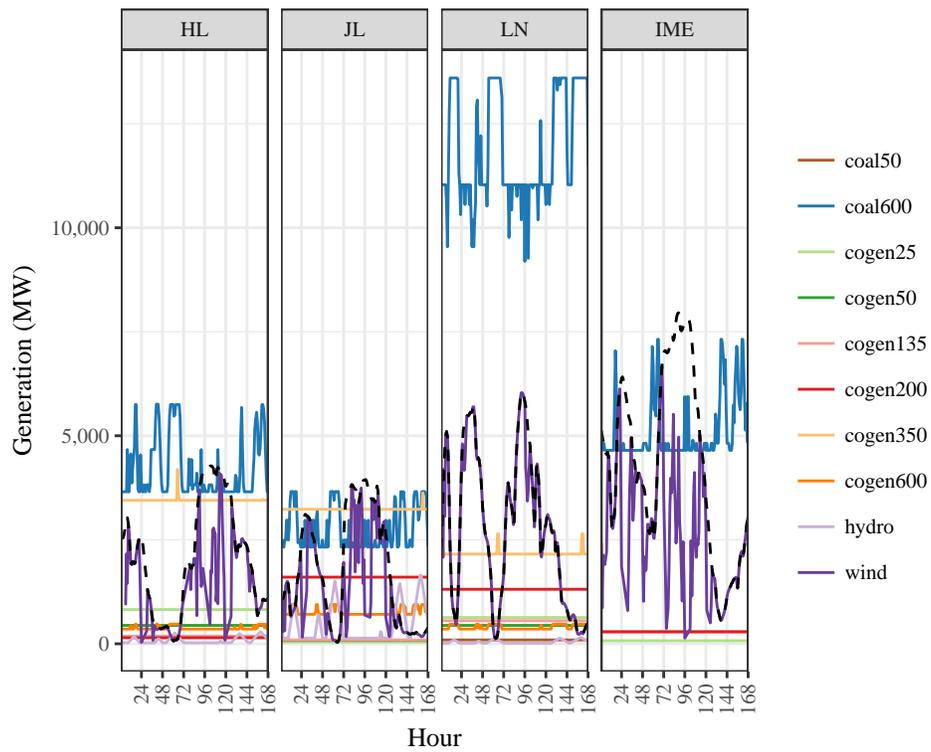
Figure 5.6: Single week generation profile for one wind scenario in the reference case, Northeast. Dotted lines are pre-curtailment wind. (full reserves)
