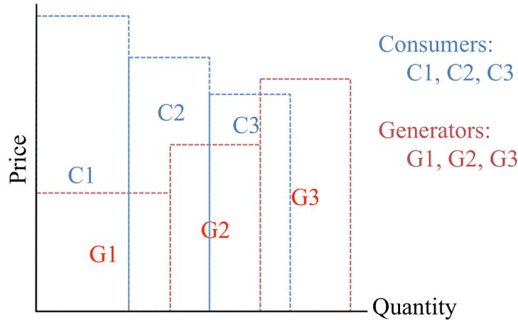
Figure 3.12: Example set of consumer and generator bids in dual-sided centralized auction
