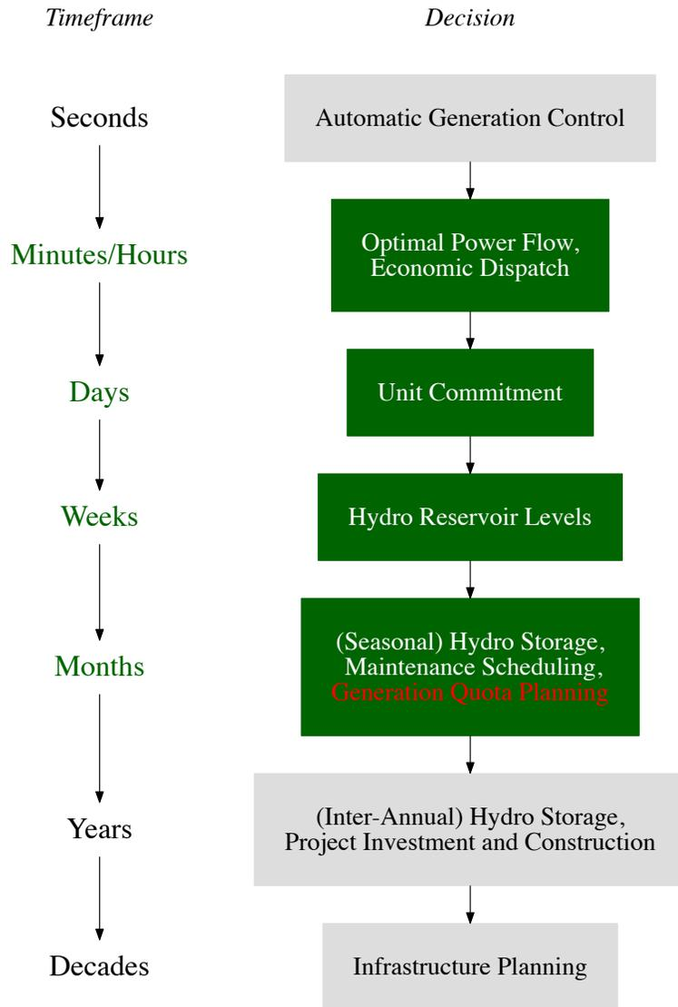
Figure 4.1: Overview of typical grid decisions and timeframes (red indicates Chinese system-specific). Dark shaded are the focus of this dissertation. Modified from: (Momoh, 2009).
