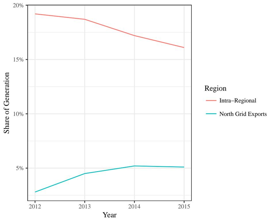
Figure 3.8: North Grid and intra-regional exports in Northeast Grid, 2012-2015. Source: author's calculations based on State Grid exchange reports.
