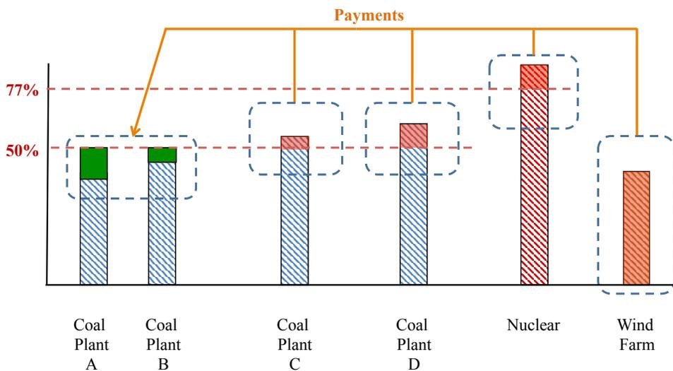
Figure 3.10: Northeast peaking ancillary services market system of payment transfers. Coal plants A and B are generating below their minimum output, and thus will receive payments from coal plants C and D, the nuclear plant and the wind farm. These payments will scale with the amount these generators' outputs exceed their minimum outputs which varies by type. The precise coal plant thresholds (here, 50%) vary by season, see Table 3.7. Source: (NEA, 2014b; Northeast ERO, 2016).
