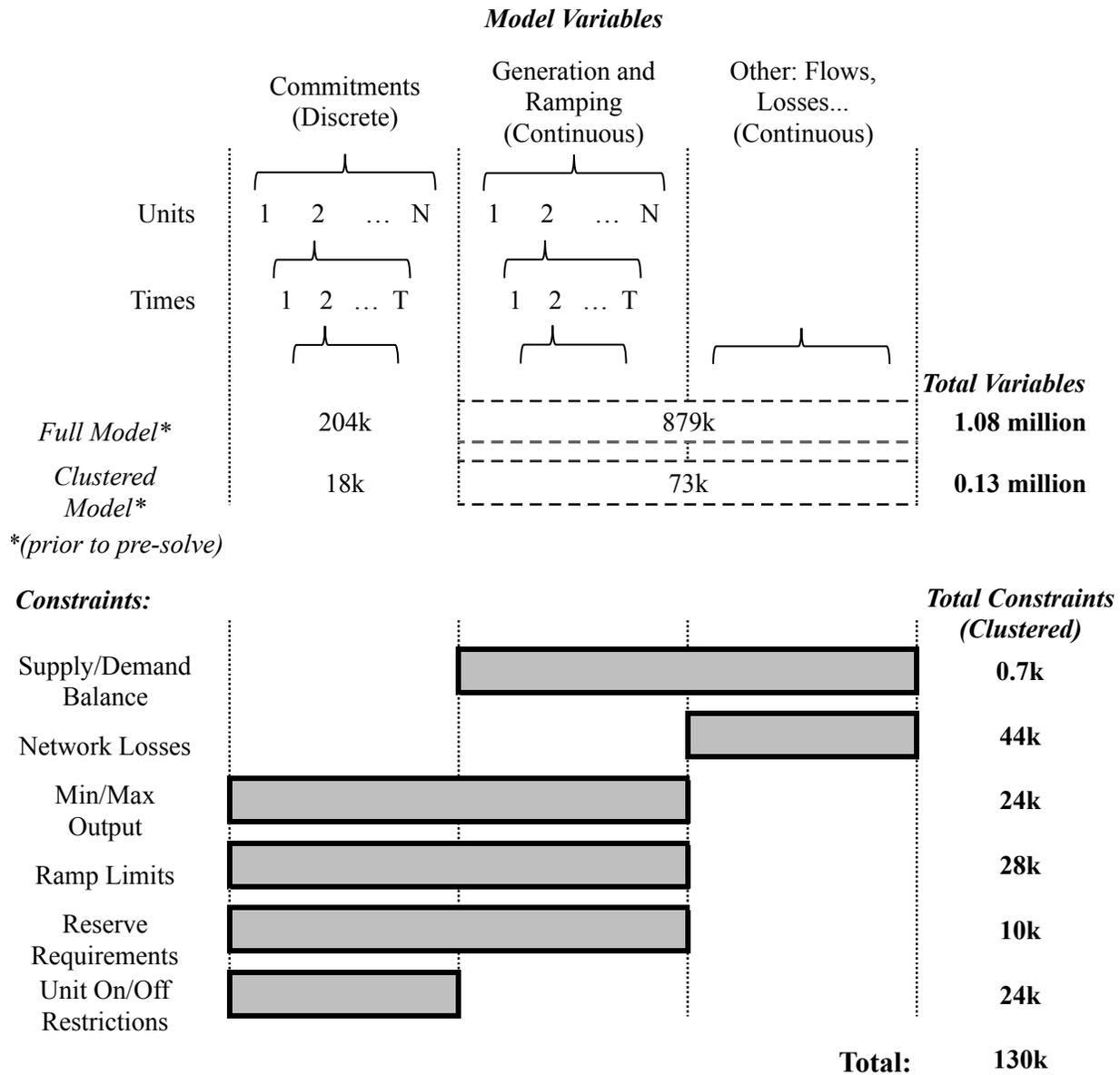
Figure 4.2: Structure of variables and constraints in unit commitment (UC) model. Blocks under constraints indicate which variables are included in equation systems. Totals shown here are for the Northeast 2011 system. Full Model:  $N = 492$ ,  $T = 168$ . Clustered Model:  $N = 4 \cdot 12 = 48$  (# provinces x # clusters),  $T = 168$ .
