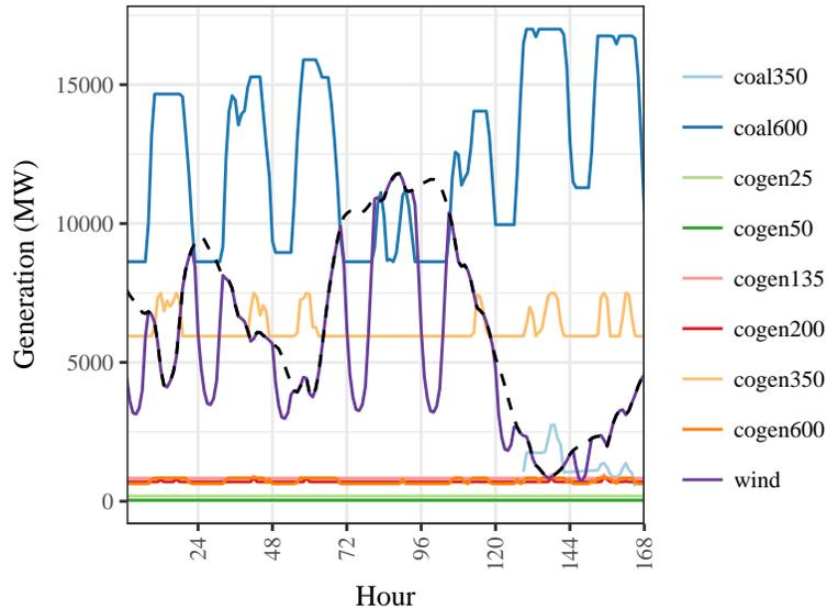
Figure 5.22: A single week’s generation profiles in the reference case, W. IM. Dotted line indicates pre-curtailment wind. (15Ja1 wind profile)
