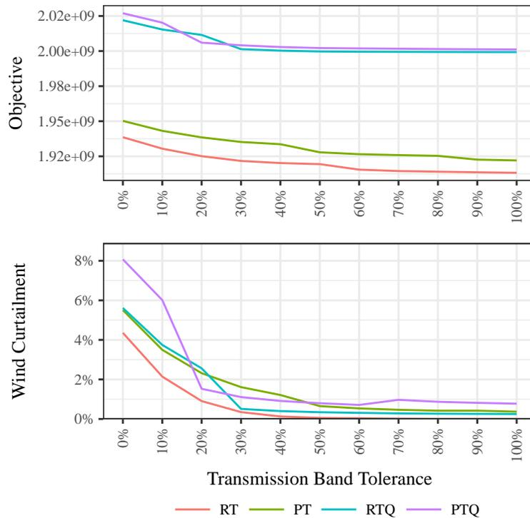
Figure 5.38: Objectives and wind curtailment for *Min Wind* commitments and transmission band tolerance sensitivity, Northwest.
