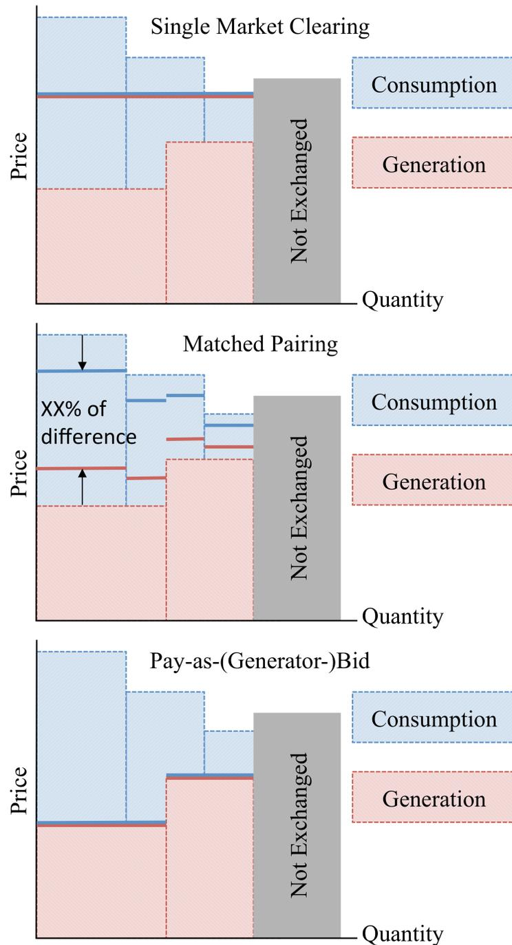
Figure 3.13: Three price formation processes for centralized dual-sided auctions. In matched pairing, the percent of the difference returned each to generators and consumers varies: e.g., 10% in Yunnan day-ahead and 50% in Guangdong monthly. Sources: (YN IIC, 2017; North China ERO, 2016b; GD EIC, 2016).
